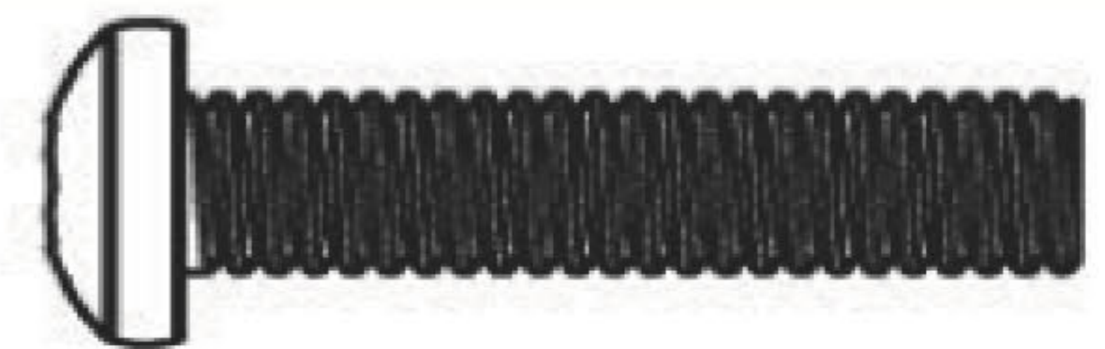
Part No.14 Round Head Bolts 3/8" x 1 1/2"
